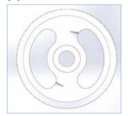
New left and right pump dedicated distributors have been defined making a niche of specific compensation. The cam pin was taken back to the centre with stamping of the displacement. (Below an example for distributor 108 cc - right)
