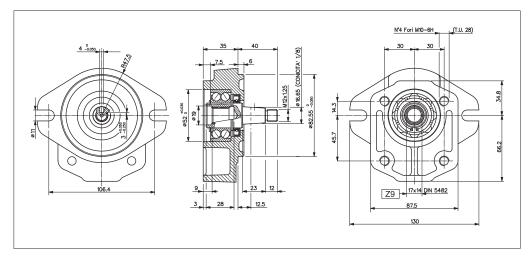
The SU/SAEA-R is suitable for driving non-standard Gr. 2 pumps and motors with belts, chain or other transmission, in which heavy combined loads take place (axial and radial)
