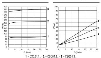
Fluid used: mineral based oil with viscosity 32 mm<sup>2</sup>/s at 40°C.
